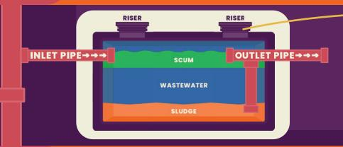
Wastewater should be at 8-10". If your wastewater level is less than 8 inches from the top of the inspection pipe, call ACE!
