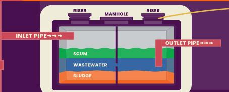
There should be an air gap of 8" - 10" between the top of the tank and the wastewater. If your wastewater level is less than 8 inches from the top of the inspection pipe, call ACE!
